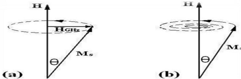
**Figure (2.5): Precessional motion of magnetization: (a) precession maintained by an applied microwave field  $H \text{ GHz}$ ; (b)  $M_s$  spiraling into line with  $H$  as the precessional energy is dissipated [48].**
