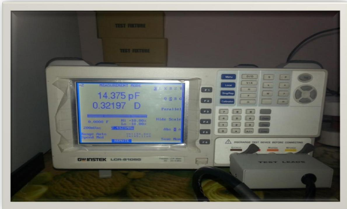
**Figure (3.8) LCR meter used in electrical measurement**
